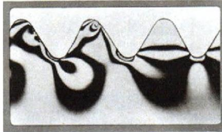
**JOINT UNDER STRESS.** This is a picture of stress patterns along the threads of a pipe joint. Crowding of lines at roots of threads indicates stress concentrations. "Three-dimensional photo-elastic stress analysis," done in U.S. Steel laboratories, helps to assure strong joints between sections of U.S. National Pipe used in drilling for oil.
