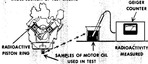
**HOW RADIOACTIVITY TEST WORKS:** motor oil used in test runs picks up microscopic metal particles worn from radioactive piston ring. Radioactivity of oil sample, measured by a Geiger counter, shows rate of engine wear. (Don't worry—the motor oil you buy is not radioactive.) Tests show today's motor oils can actually triple life of your car engine.
